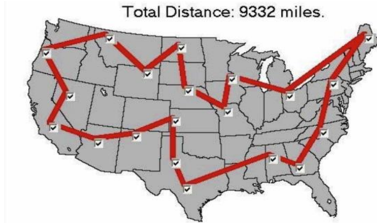
Figure 2: The TSP Solution for a 20-City Problem Having 6.1 \times 10^{16} Permutations (from http://www.solver.com/solver-platform-sdk-source-code-examples )
